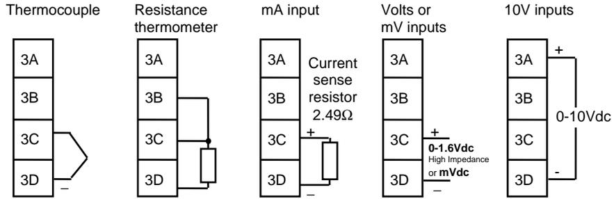
Figure 1-8 Connections for Process Value 2 (PV2)
