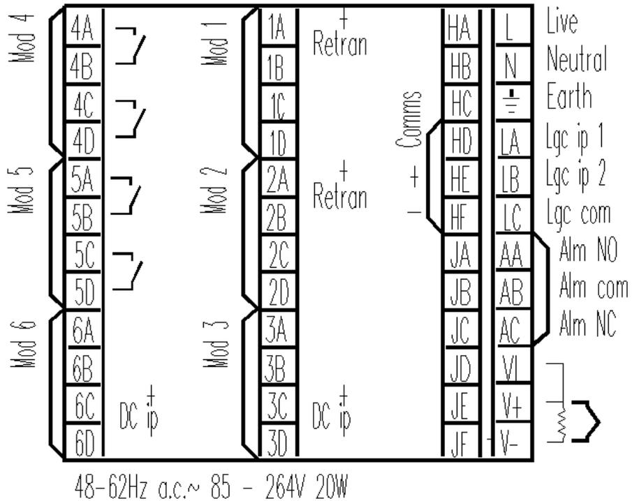
Figure 1-6 Rear terminal layout
