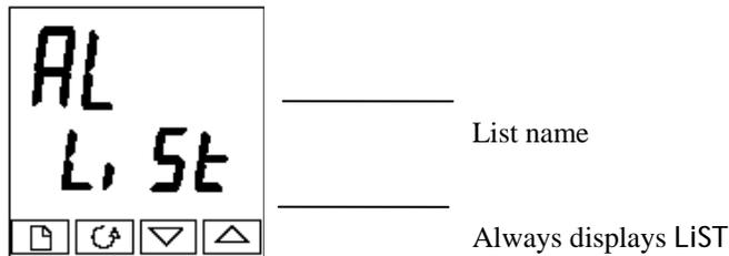
Figure 2-5 Typical list header display
