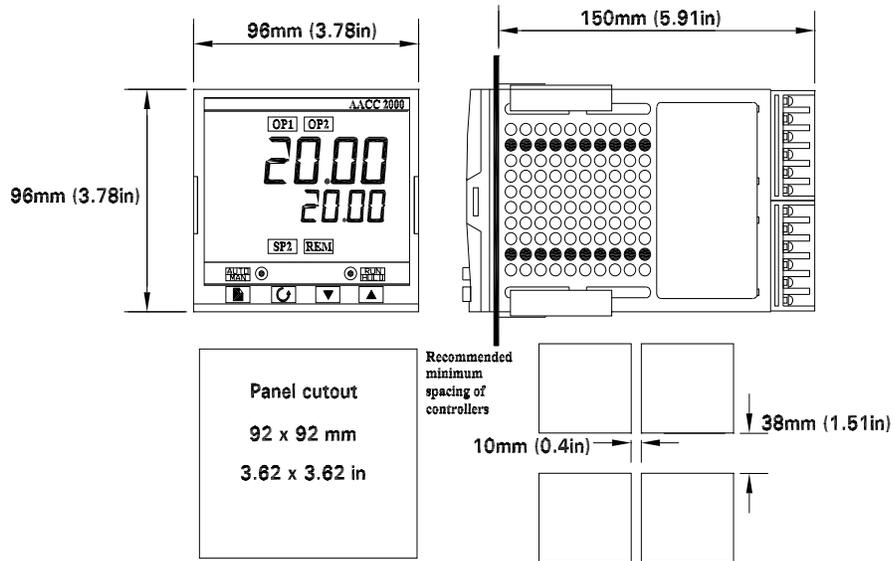
The electronic assembly of the controller plugs into a rigid plastic case, which in turn fits into the standard DIN size panel cut-out shown in Figures 1-3 and 1-4.
