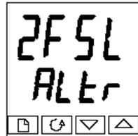
The parameter selected is the sepoint for Alarm 2 - Full Scale Low
