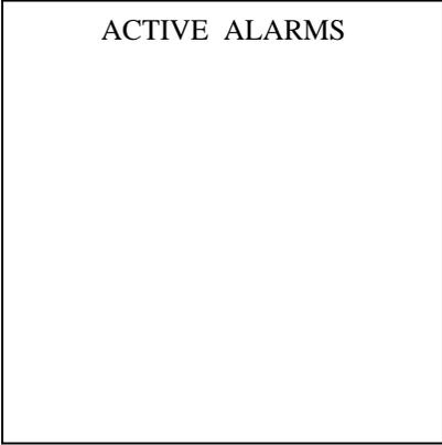
This screen will display messages for any and all active alarm conditions. Use the knob to scroll through the messages if the screen is full. Active alarms will automatically clear from this screen when conditions change.
