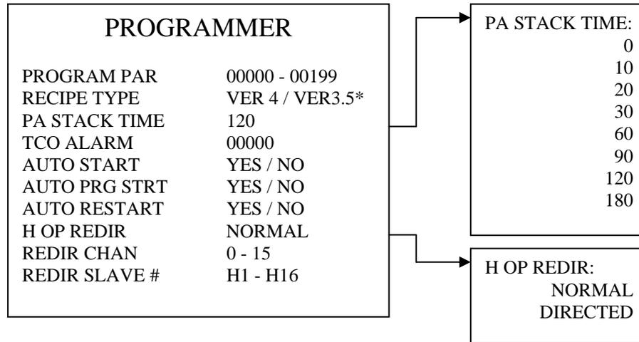
This screen is used to setup parameters related to logic programs.
