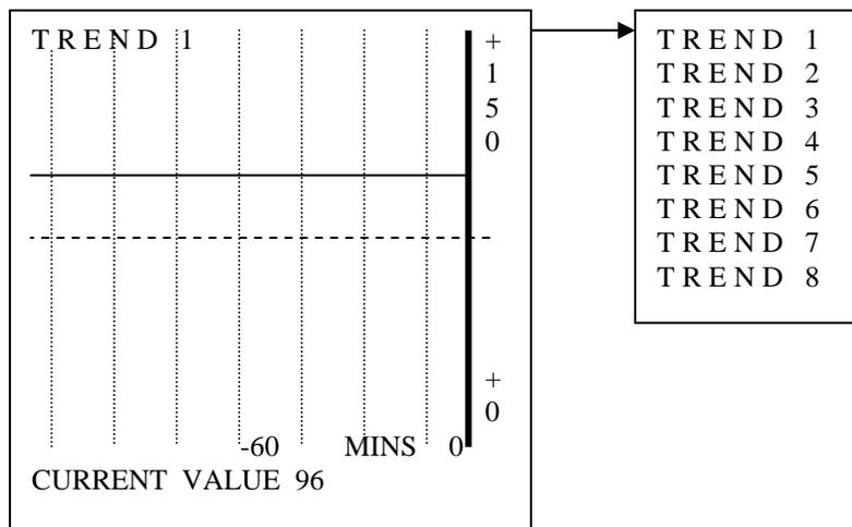
These screens show the trend data stored in the instrument. The knob can be used to scroll back and view older data. Near the bottom of the screen is the current data and relative time in minutes. The numbers on the right define the scaling range of the grid. The message title at the top can be changed with the text entry screen. Pressing the knob jumps to the trend zoom screen for the trend. The zoom allows up to a 20 to 1 compression of the time.
