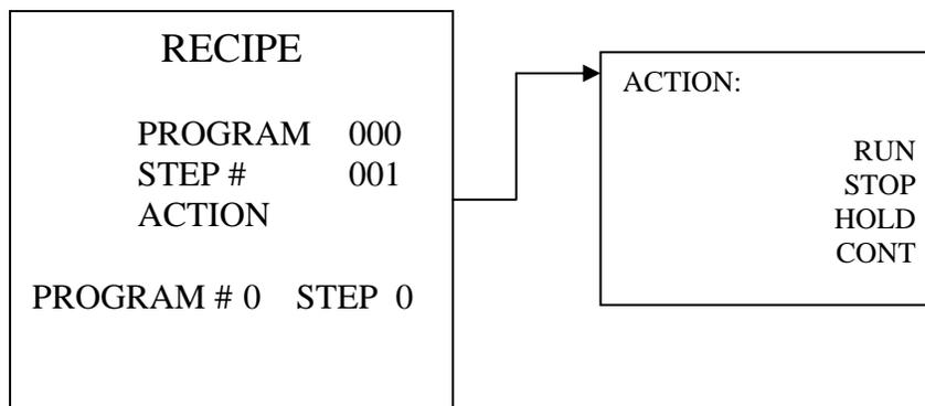
The operator can run / stop / hold / continue any recipe in the instrument.
