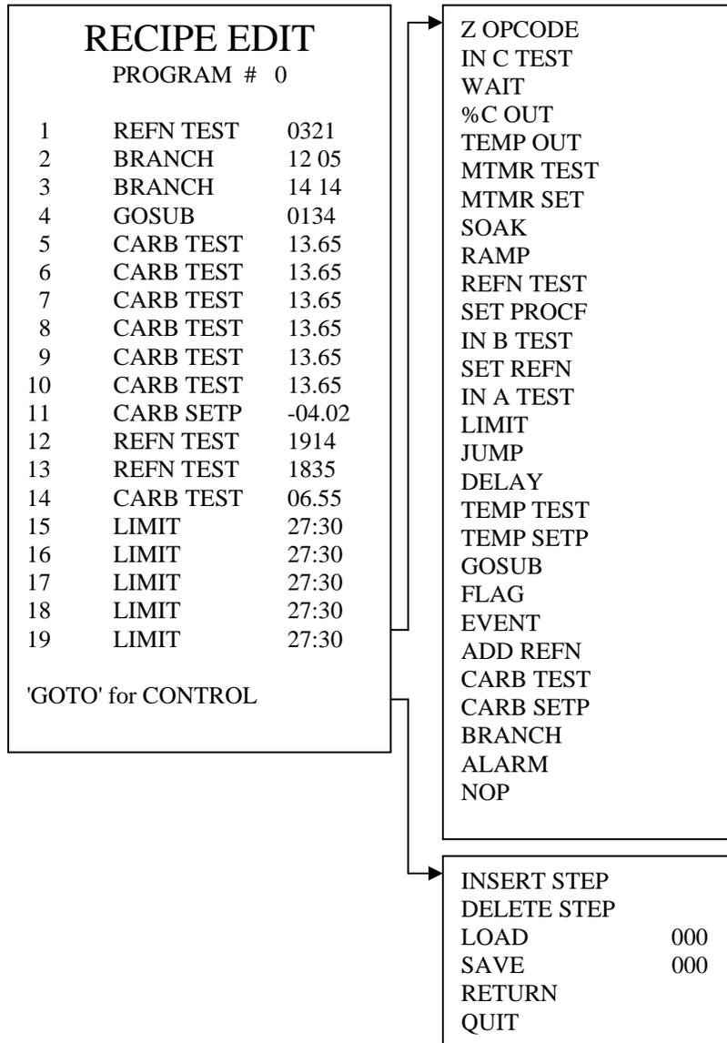
Pressing the 'GoTo' key provides a selection of edit and control features.
