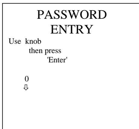
This screen is used to set the password. A password is always required to enter this screen.
