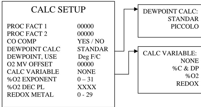
Process factor can be entered to adjust carbon potential calculation.
