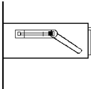
[To prevent damage or warping of the unit's case, **do not** over tighten the clamp bolts.]
