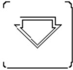
This key is usually used to decrease the value of a digit in the data entry mode or scroll through various parameter sequences. In Manual mode this key will cause the control action to move toward the Output 2 direction. When used in the dual-key operation Shift/"down arrow" it accesses the Programmer Status Display.
