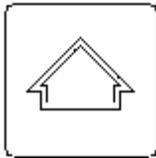
This key is usually used to increase the value of a digit in the data entry mode or scroll through various parameter sequences. In Manual mode this key will cause the control action to move in the Output 1 direction. When used in the dual-key operation Shift/"up arrow" an LED test is activated, where every segment and decimal point should light in both displays. If any segment or decimal point does not light a keyboard problem may exist, contact a qualified MMI representative.
